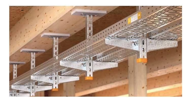
Perforated fire protection plate as effective panelling measure for fastening on supporting wooden components for the maintenance of electrical function according to DIN 4102 Part 12. Made of fibre-glass lightweight concrete, which is resistant to water and frost (material class A1 – non-combustible)
