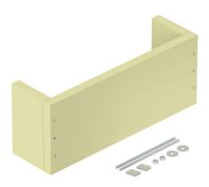
Strain relief as an effective support measure for vertical cable routing, according to DIN 4102 Part 12. Approved for all cable types and all vertical routing systems, which are mounted directly on solid walls. Maintenance of electrical function classes E30 to E90. Empty housing for individual filling with the PYROSIT® NG fire protection foam and/or PYROPLUG® Block insulation systems, incl. mounting set and labelling panel.
