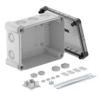
Junction box with hat profile rail for the connection of cables and lines indoors and in outdoor areas. Rectangular design with knock-out entries. Suitable for wall and ceiling mounting with the option to fasten outside, inside or to mount via the corner domes. Particularly impact resistant with IK09. Transparent cover with quick lock, sealable. Made from halogen-free and UV-resistant materials.
