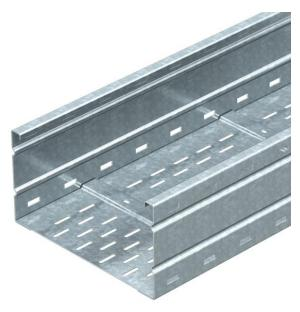
Wide span cable tray system, perforated, with a side height of 160 mm. Straight connectors of type WRV 160 should be ordered separately and in the appropriate quantity.
