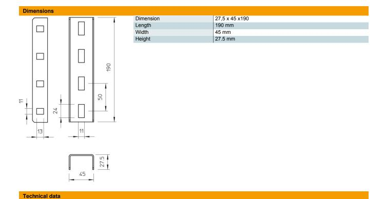
Drill hole spacing, centre Suitable for profile shapes
