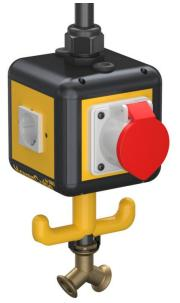
Housing equipped and pre-wired, with 1 m pipe 1/2" and connection for compressed air hose 13 x 3.5 mm and 2-way distributor 1/2", with suspension lug, grip hook and four cover plates.
