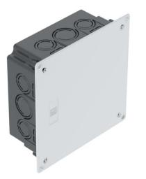
Flush-mounted connection box for clamping terminals, for use in masonry with an installation depth of at least 65 mm. With cover and cover screws (15 mm). Flat cover edge, roughened surface.
