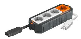
The ready-for-connection UTC4 universal support possesses 3 pre-installed 33° protective contact sockets in white and 1 pre-installed 33° protective contact socket in orange (with surge protection module, type 3, according to DIN EN 61643-11), 250 V~, 16 A. Suitable for VL connection cables and device installation units of nominal size R7, R9 and 9.
