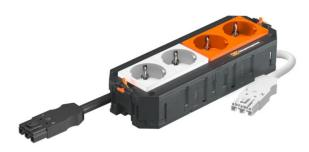
The ready-for-connection UTC4 universal support possesses 2 pre-installed 33° protective contact sockets in white and 2 pre-installed 33° protective contact sockets in orange (with surge protection module, type 3, according to DIN EN 61643-11), 250 V~, 16 A. Suitable for VL connection cables and device installation units of nominal size R7, R9 and 9.
