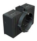
Device/connection socket with increased socket volume on both sides of the device installation opening to accept connection terminals. Torsion-resistant guaranteed standard combination spacing of 71 mm (to DIN 49 073-1) through snap—lock coupling. Break-out openings for cables and pipes of up to  $\emptyset$  21 mm, low-lying plaster brackets,
