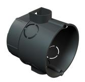
Device/connection socket with torsion-resistant guaranteed standard combination spacing of 71 mm (to DIN 49 073-1) through Snap–lock coupling. Break-out openings for cables and pipes Ø 20 mm and Ø 25 mm. Combinable for spreading and screw fastening, low-lying plaster brackets, device bolt spacing 60 mm, for screw fastening with 3.2 mm self-tapping screws, with 2 screw bosses without screws, protection rating IP20.
