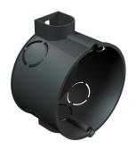
Device socket with torsion-resistant guaranteed standard combination spacing of 71 mm (to DIN 49 073-1) through Snap–lock coupling. 7 break-out openings for cables and pipes  $\varnothing$  20 mm and  $\varnothing$  25 mm. Combinable for spreading and screw fastening, low-lying plaster brackets, device bolt spacing 60 mm, for screw fastening with 3.2 mm self-tapping screws, with 2 screw bosses without screws, protection rating IP20.
