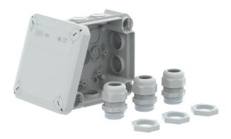
Junction box for the connection of cables indoors and in protected outdoor areas. Square design with plug-in seals to the sides and knock-out entries in the bottom. Suitable for wall and ceiling mounting and on mounting panels. With the option of fastening inside and to mount via the corner domes. Cover with quick lock, sealable. Made from halogen-free and UV-resistant materials.
