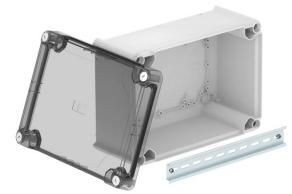
Closed junction box for the connection of cables and lines indoors and in protected outdoor areas. Rectangular design without entries. Suitable for wall and ceiling mounting, on mounting panels and threads in the floor. With the option to fasten inside and to mount via the corner domes. High, transparent cover with quick lock, sealable. Made from halogen-free and UV-stabilized materials.
