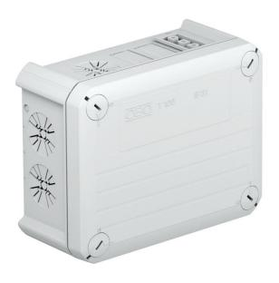
Junction box with Wieland sockets, 1w3p + 1s3p, for the connection of cables indoors and in protected outdoor areas. Rectangular design with knock-out entries to the sides and knock-out entries in the bottom. Suitable for wall and ceiling mounting and on mounting panels. With the option of fastening inside and to mount via the corner domes. Cover with quick lock, sealable. Made from halogen-free and UV-resistant materials.
