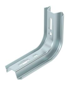
TP support/bracket for fastening to horizontal concrete ceilings and walls. If the profile is fastened directly to the ceiling or the profile is screwed together as head reinforcement, then, for reasons of stability, always use the spacer, type DS 4.
