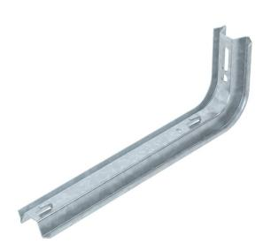
TP bracket with clamping lugs. If the bracket is fastened directly to the wall or the profiles are screwed together, then, for reasons of stability, always use the spacer, type DS 4. Mesh cable trays with a 50 x 100 mm grid width, e.g. type GRL, GR and GRM, can be fastened to the TP bracket without screws.
