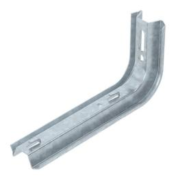
TP bracket with clamping lugs. If the bracket is fastened directly to the wall or the profiles are screwed together, then, for reasons of stability, always use the spacer, type DS 4. Mesh cable trays with a 50 x 100 mm grid width, e.g. type GRL, GR and GRM, can be fastened to the TP bracket without screws.
