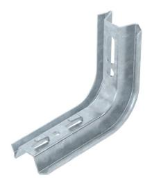
TP bracket with clamping lugs. If the bracket is fastened directly to the wall or the profiles are screwed together, then, for reasons of stability, always use the spacer, type DS 4. Mesh cable trays with a 50 x 100 mm grid width, e.g. type GRL, GR and GRM, can be fastened to the TP bracket without screws.
