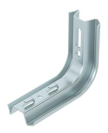
TP bracket with clamping lugs for screwless mesh cable tray fastening. If the bracket is fastened directly to the wall or the profiles are screwed together, then, for reasons of stability, always use the spacer, type DS 4. Mesh cable trays with a 50 x 100 mm grid width, e.g. type GRL, GR and GRM, can be fastened to the TP bracket without screws.
