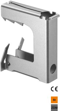
The multifunctional beam clamp is suitable for fastening cables, protective pipes and cable sections on steel girders of any size (one clip for every application). Here, the beam clamp is very versatile thanks to various fastening options. Mounting of the beam clamp is quick and efficient, with no need for welding or drilling. It is simply mounted by hammering or pushing into place. The beam clamp can be used in both internal and external areas.
