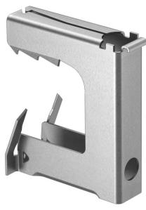
The multifunctional beam clamp is suitable for fastening cables, protective pipes and cable sections on steel girders of any size (one clip for every application). Here, the beam clamp is very versatile thanks to various fastening options. Mounting of the beam clamp is quick and efficient, with no need for welding or drilling. It is simply mounted by hammering or pushing into place. The beam clamp can be used in both internal and external areas.
