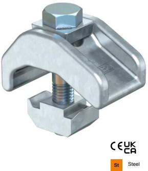
Heavy-duty chuck jaw with slide nut for fastening profile rails to steel girders. The clamping range of the chuck jaw is limited to the maximum fastening thickness, 30 mm.
