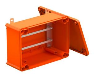
Unequipped, closed connection or junction box for free termination with ceramic terminals and cable glands. Dimension A states the available support rail length for the wiring terminals. Sufficiently large wiring compartment through diagonally arranged support rail. Fastening on easily accessible external flaps made of stainless steel. Approved for cable systems that maintain the electrical function according to DIN 4102 Part 12 with the classes E30, E60 and E90.
