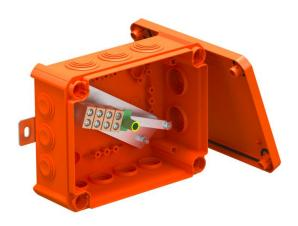
Connection box with soft plug-in seals. Sufficiently large wiring compartment through diagonally arranged connection unit with completely pre-mounted, high-temperature-resistant ceramic terminals. Green-yellow labelled protective conductor terminal. Fastening on easily accessible external flaps. Approved for cable systems that maintain the electrical function according to DIN 4102 Part 12 with the classes E30, E60 and E90. Ceramic clamps have been tested according to DIN EN 60998-2-1:2004.
