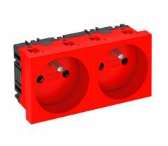
Socket with earthing pin, double  $0^\circ,$  with increased touch protection, with screwless terminals, 2-pin, 16 A, 250 V~, with connection terminals to IEC 60884-1.
