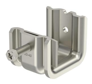
This type of beam clamp is pushed onto the support and fixed to the girder or flat iron using a pressure trough and bolt (M8). The hexagonal bolt has a WAF of 10 mm. In the clip element, two additional M6 threads are also incorporated, to fix threaded rods, for example.
