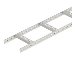
Shipbuilding cable ladder with perforated side rail of side height 40 mm with wel-ded, perforated trapezoidal rungs which open in a downwards direction. Load tested according to IEC in conjunction with connector, type SLV. The shipping cable ladder is also available in unpainted steel on request.
