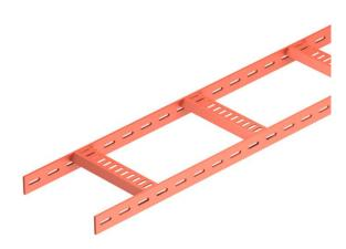
Shipbuilding cable ladder with perforated side rail of side height 40 mm with welded, perforated trapezoidal rungs which open in a downwards direction. Load tested according to IEC in conjunction with connector, type SLV. Welding primer type SIGMA-WELD 199.
