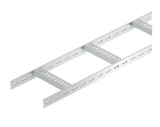
Shipbuilding cable ladder with perforated side rail of side height 40 mm with welded, perforated trapezoidal rungs which open in a downwards direction. The shipbuilding cable ladder is also available in unpainted steel on request.
