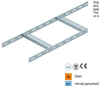
Shipbuilding cable ladder with perforated side rail of side height 25 mm with wel-ded, perforated trapezoidal rungs which open in a downwards direction. Load tested according to IEC in conjunction with connector, type SLV. The shipbuilding cable ladder, including fittings, is also available in stainless steel on request. Powder coating according to RAL colours possible.
