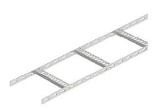
Shipbuilding cable ladder with perforated side rail of side height 25 mm with welded, perforated trapezoidal rungs which open in a downwards direction. Load tested according to IEC in conjunction with connector, type SLV. The shipbuilding cable ladder is also available in unpainted steel on request.
