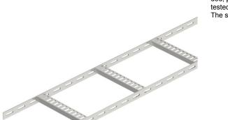
Shipbuilding cable ladder with perforated side rail of side height 25 mm with wel-ded, perforated trapezoidal rungs which open in a downwards direction. Load tested according to IEC in conjunction with connector, type SLV. The shipbuilding cable ladder is also available in unpainted steel on request.
