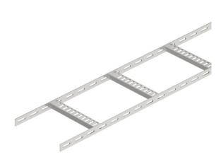
Shipbuilding cable ladder with perforated side rail of side height 25 mm with welded, perforated trapezoidal rungs which open in a downwards direction. Load tested according to IEC in conjunction with connector, type SLV.
