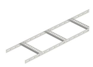
Shipbuilding cable ladder with perforated side rail of side height 25 mm with welded, perforated trapezoidal rungs which open in a downwards direction. Load tested according to IEC in conjunction with connector, type SLV.
