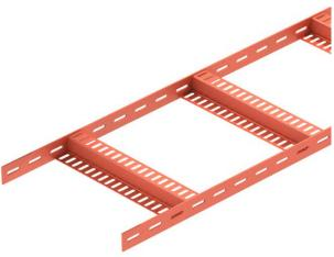
Light-duty shipbuilding cable ladder with perforated side rail of side height 35 mm with welded, perforated Z rungs. Load tested according to IEC in conjunction with connector, type SLV. Welding primer type SIGMA-WELD 199, also available in white
