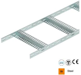
Light-duty shipbuilding cable ladder with perforated side rail of side height 35 mm with welded, perforated Z rungs. Load tested according to IEC in conjunction with connector, type SLV.
