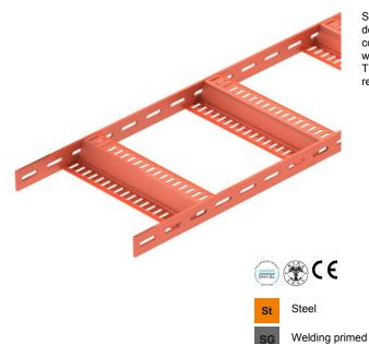
Shipbuilding cable ladder with perforated side rail of side height 40 mm with welded, perforated Z rungs. Load tested according to IEC in conjunction with connector, type SLV. Welding primer type SIGMA-WELD 199, also available in white.
