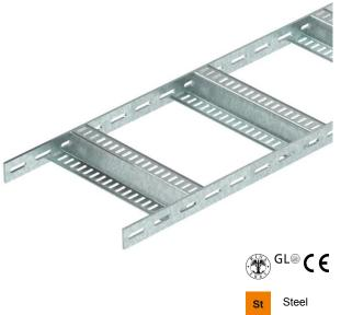
Shipbuilding cable ladder with perforated side rail of side height 40 mm with welded, perforated Z rungs. Load tested according to IEC in conjunction with connector, type SLV.
