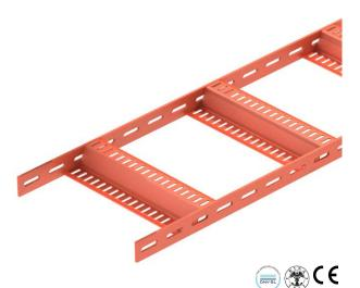
Shipbuilding cable ladder with perforated side rail of side height 40 mm with welded, perforated Z rungs. Load tested according to IEC in conjunction with connector, type SLV. Welding primer type SIGMA-WELD 199, also available in white.
