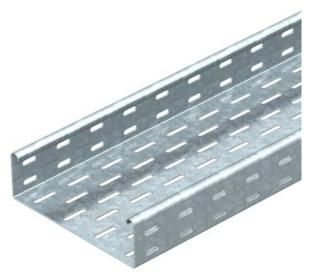
SKS 60 = Heavy-duty cable tray system with 60 mm side height. The cable tray, type SKS, should also be used for the maintenance of electrical function. For additional data, please refer to BSS fire protection systems. Magnetic shield insulation without cover 20 dB, with cover 50 dB.
