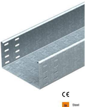
SKS 110 = heavy-duty cable tray system, unperforated, with 110 mm side height. The cable tray has connector perforations on both sides. Straight connectors should be ordered separately and in the appropriate quantity. Magnetic shield insulation without cover 20 dB, with cover 50 dB.
