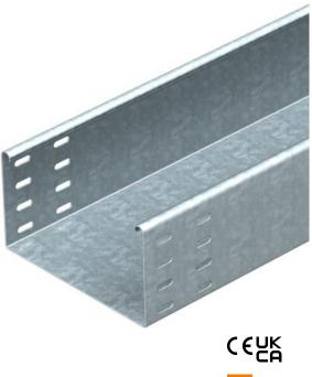
SKSU 110 = heavy-duty cable tray system, unperforated, with 110 mm side height. The cable tray has connector perforations on both sides. Straight connectors should be ordered separately and in the appropriate quantity. Magnetic shield insulation without cover 20 dB, with cover 50 dB.
