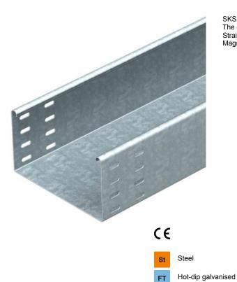
SKS 110 = heavy-duty cable tray system, unperforated, with 110 mm side height. The cable tray has connector perforations on both sides. Straight connectors should be ordered separately and in the appropriate quantity. Magnetic shield insulation without cover 20 dB, with cover 50 dB.
