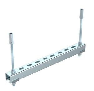
Suspension and fastening material, made of steel, to create the first support of pass-through installations in fire insulation. Mounting of the pendulum with threaded rods under the ceiling. A maximum of two layers can be mounted with connection sleeves from two sets. The support constructions must be arranged on both sides of the wall at the prescribed distance to the insulation system. Including 2x MMS-plus I 7.5 x 40
