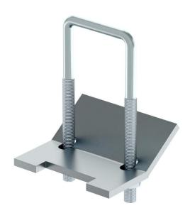
Connection element for two-sided fastening of profile rails to steel girders. Fastening is possible independently of the arrangement of the rail opening. The rail length should be at least the width of the steel girder + 2 x 50 mm. Always use in pairs for mounting. For use with profile rail MS4022, MS4141, MS4142, MS4124.
