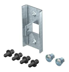
Rung seat for fastening rungs of type MS4022 to steel girders. The set consists of two rung seats, two hexagonal bolts M8 x 16 mm and four hexagonal bolts with an M10 x 30 application tip.
