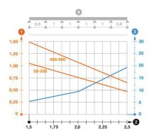
Load diagram, cable tray, type RKS 60, unbeaded
