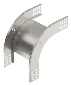
90° vertical bend, falling, for all cable tray types of 60 mm side height. The vertical bend is pushed over the end of the cable tray and screwed tight. Fastening materials should be ordered separately.
