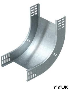
90° rising vertical bend, for all cable tray types of 60 mm side height. The vertical bend is pushed over the end of the cable tray and screwed tight. Fastening materials should be ordered separately.
